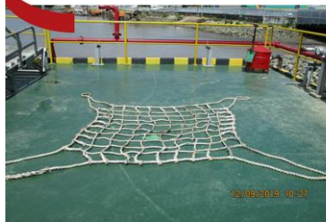
Applied net for lifting equipment from ship Copyright of Shell International
