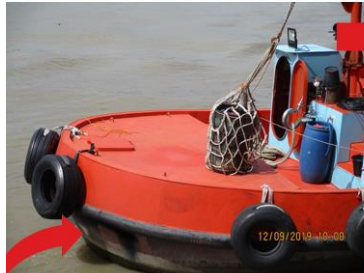
Secured equipment by net prior lifting
